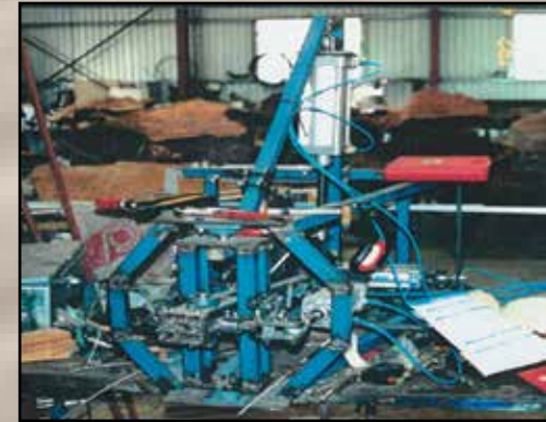
Robotic Dinosaur Internal Steel Frame
