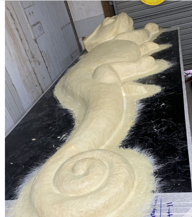
Applying fibreglass to the mould
