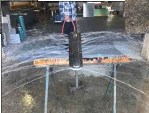
Front View with water - spraying under pressure
